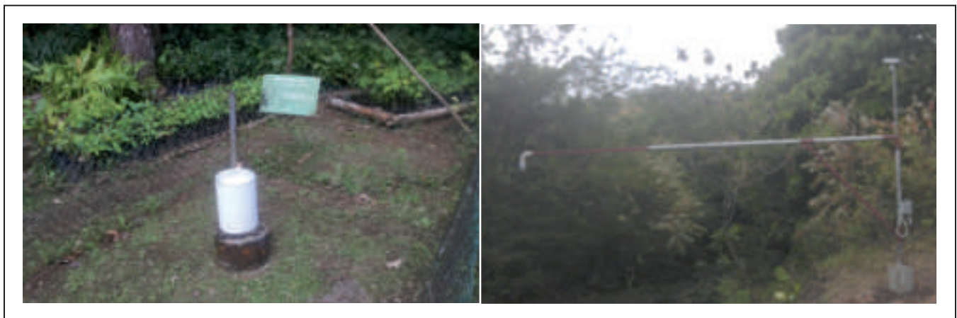
Rainfall logger at Barre de l'Isle (left) and water level recorder in Dauphin watershed (right)
