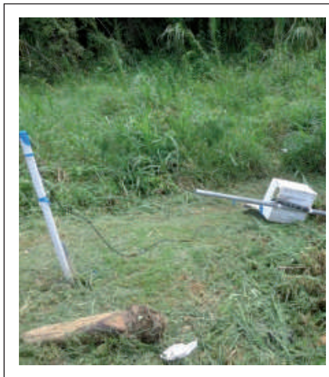
Vandalized hydro-met equipment
